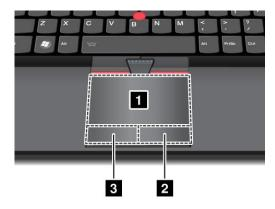
Movement on the touch pad emulates operations on the mouse. Before interacting with the touch pad, make sure the cursor stays on the object that you want to operate.
